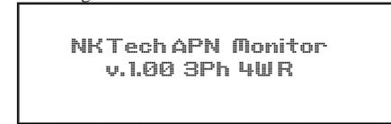
Product series, firmware version, and meter configuration (three phase, four wire). "R" refers to RC current inputs
