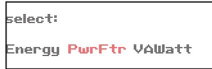
The power factor is shown with a (+) positive notation for inductive loads, and a (-) notation for loads which are capacitive. If the monitored load is inductive, all three phases should show power factor as positive. A negative value will be displayed if the load is capacitive.
