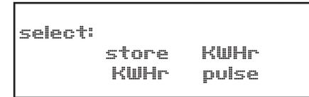
3. Select "Store KWHr" to save the accumulated watt hour value to flash memory. The count will be restored after a loss of power. Select "KWHr Pulse" to save the counts to the Energy display only (lost is power is interrupted). Select either to set the pulse interval for watt hour counting. Pressing "KWHr Pulse" before "Store KWHr" will clear any previously accumulated watt hour value from memory.
