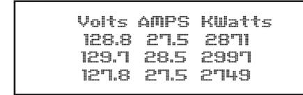
Voltage and current are RMS values, the watts displayed are active power.
