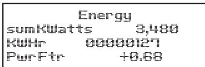
Sum KWatts shows the active power being used at any time. KWHR increases as kilowatt hours are accumulated. Pwr Ftr shows the average power factor of all three phases.
