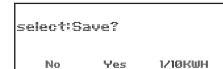
Press the "Yes" button to set the pulse rate (1/10KWH) one pulse per ten kilowatt hours. This is the available option with this model. The solid state no voltage contact will open and close when 10 kilowatt hours have accumulated.
