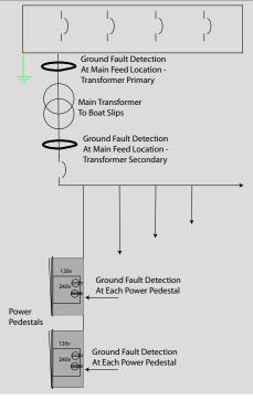
The diagram above illustates the wiring of a sensor for ground fault detection in marinas.
