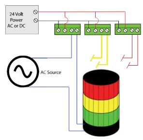
Example of three ASD switches powered from one supply, so when current through one of the switches reaches setpoint the output closes to energize one level of the stack light.
