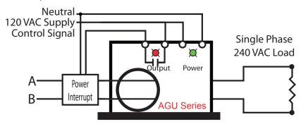
Three-phase circuits, 3-wire delta loads up to 60 Amps can fit in the AGU Series. Since the load doesn't use neutral, it does NOT pass through the aperture. Higher amperage loads require larger gauge wire which increases the wire bundle size. The AGL Series provides a larger diameter aperture when required.
