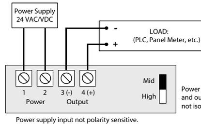
Output loop is powered by DT Transducer. No loop power supply required.
