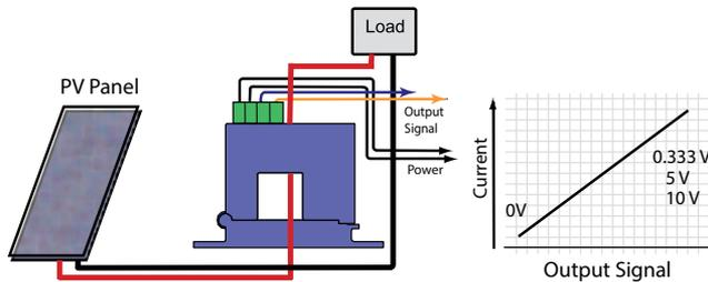
The DT sensor will produce a signal directly proportional to the current produced by the panel or string of panels, with an output to match the controller being used.
