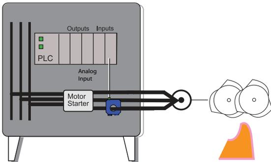
Monitor a shredding operation to measure current usage, enabling automatic shut down if the blades become jammed or overloaded.
