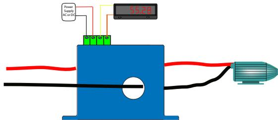
Use a DT sensor over one lead to a DC motor to measure the current used. Over normal readings mean a jam or a bearing failure, and under normal current means a belt or coupling may have broken. The output can also be used to measure time of use to help with maintenance scheduling.
