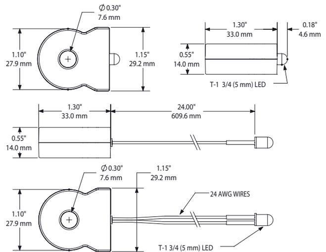
Note: Panel opening should be 0.250". Panel thickness between 0.032" – 0.125".
