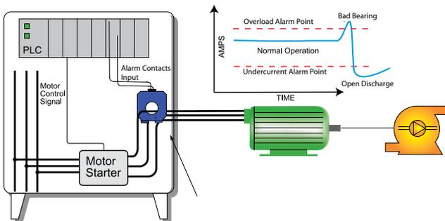
Pumps draw more current when there are mechanical problems like seizing bearings or obstructed impellers, and draw less current when the intake suction is blocked or the discharge is not connected.
