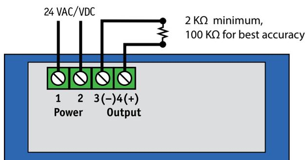
Power supply and output must be isolated.
