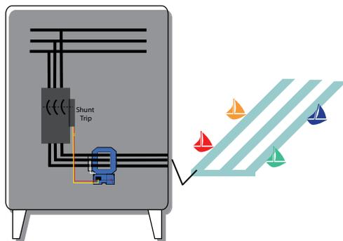
Equipment on board a vessel can pass current to earth through water, causing a dangerous condition to swimmers and boaters in fresh water marinas and boat docking facilities. Use a ground fault sensor with a shunt trip breaker to shut off the power when excessive current flows to earth.
