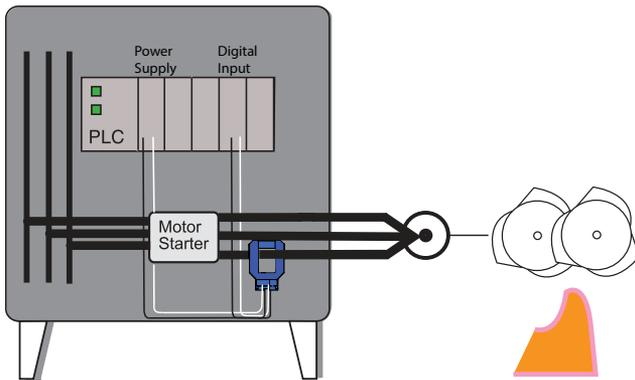
If the crusher drive draws too much current, the infeed belt can be stopped automatically, allowing the crusher to clear before restarting. The ASXP-MS provides a set of relay contacts for alarm of over or undercurrent conditions.
