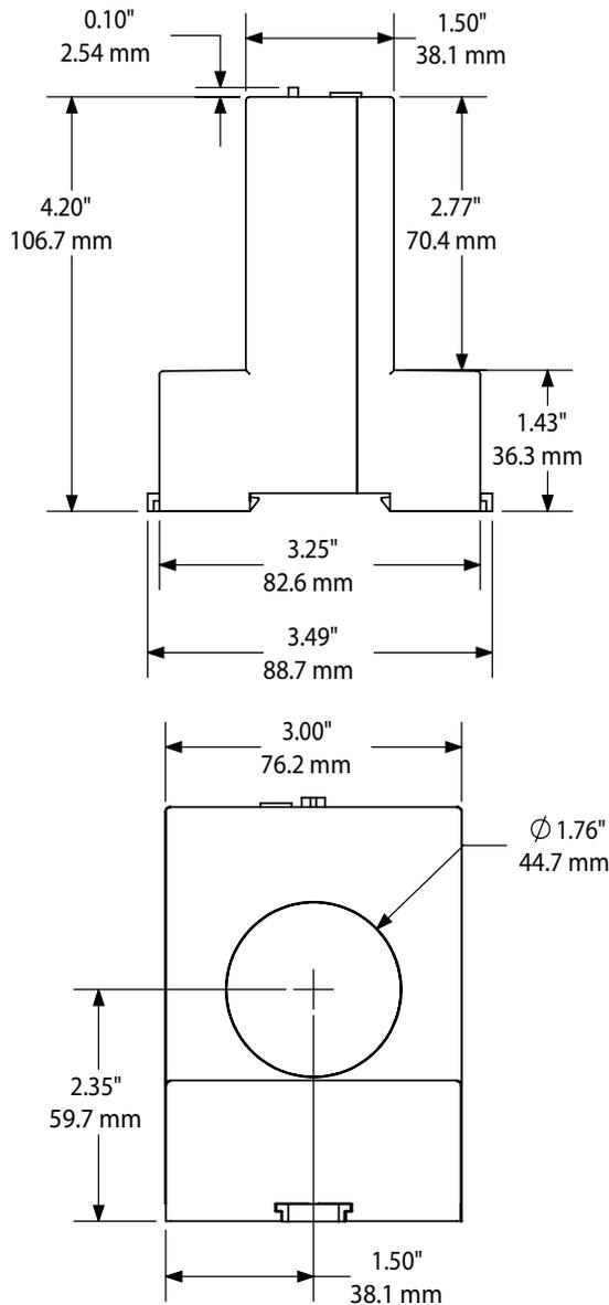
Ground Fault Relay Specifications
