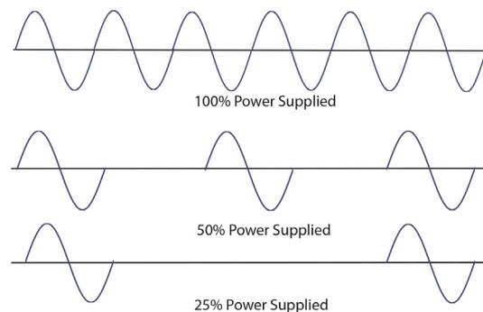
ATH AC current transducers will produce a signal proportional to the current used even when the controller is supplying power in one cycle increments. This is quite common as the “burst-fired” zero crossing switching method produces less harmonic distortion than phase-angle fired controls.
