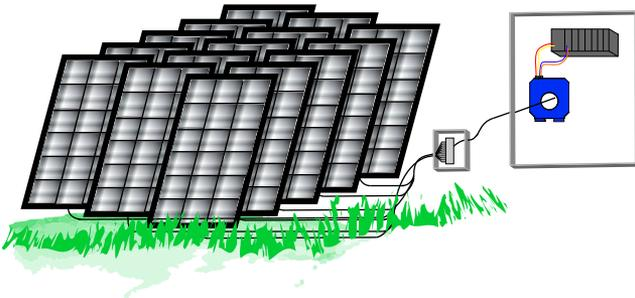
Commercial and industrial ground mounted solar arrays are connected in series to combiner boxes, developing higher voltage and lower current to deliver the same power as with a lower voltage system.
