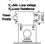
Connect the negative from the power supply to the negative of the load (panel meter, PLC, etc.). Connect the positive from the power supply to the positive terminal of the sensor. Connect the negative terminal of the sensor to the positive or input of the load.
