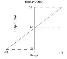
Output at mid-scale (12 mA) at zero current, 20 mA in primary direction, 4 mA in revese direction.
