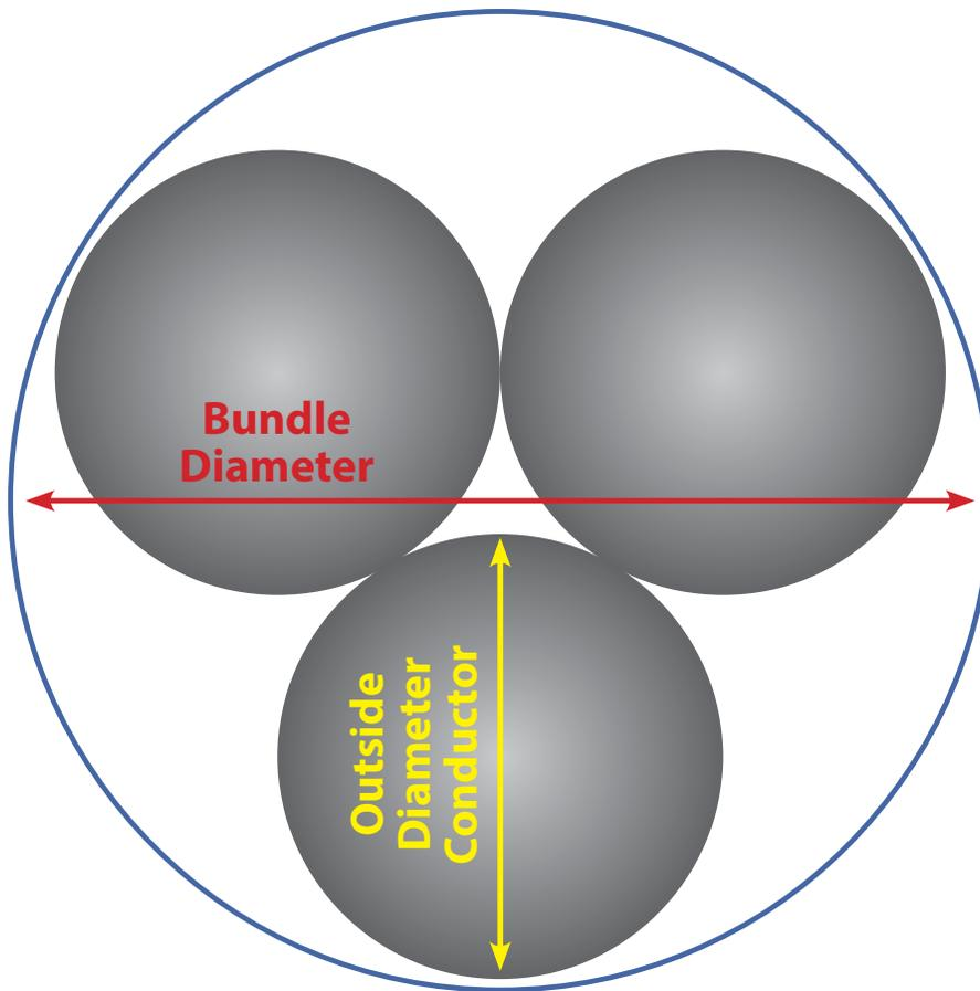
Overall wire bundle diameter is calculated using the following equation:
