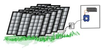
Commercial and industrial ground mounted solar arrays are connected in series to combiner boxes, developing higher voltage and lower current to deliver the same power as with a lower voltage system.
