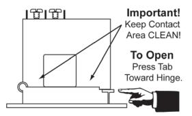
Silicone grease is factory applied on the mating surfaces to prevent rust and improve performance. Be careful not to allow grit or dirt onto the grease in the contact area. Operation can be impaired if the mating surfaces do not have good contact. Check visually before closing.
