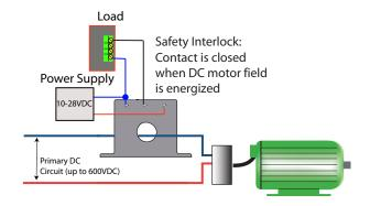
Smaller, simpler and every bit as reliable as the adjustable DS3 series, the DS1 can be used to detect even lower current levels.
