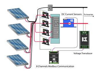
The ADC Series Analog to Digital Converter provides the perfect solution for monitoirng a photovoltaic power production system that collects input from multiple sensors.
