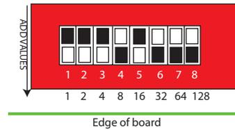
The node address is set through a series of eight dip-switches allowing a possible address range of 1-247. After converting your decimal address to binary either by hand or
