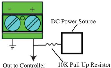
Use an external resistor of 10K ohm from the DC power to the pulse output contact (+) and out to the controller input. Ground the (-) terminal of the pulse contact. This will allow voltage to pass when the output is open, and block when closed. One kwh value is represented with an open and closed output cycle.
