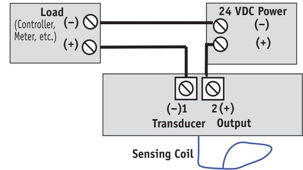
Note: The coil and the signal conditioner are matched and calibrated at the factory. If the coil is damaged in the field, please return both pieces as a set to the factory after obtaining authorization.
